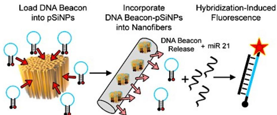
Figure 1. Hybrid polymer nanofibers containing DNA-loaded porous silicon nanoparticles allowing for long-term detection of a target microRNA.
