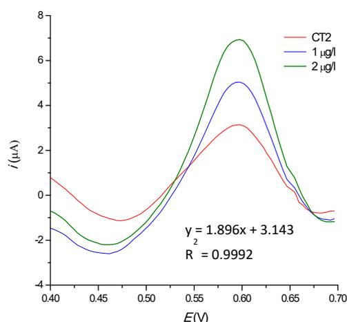
Figure 1. Voltammograms obtained for Hg quantification in a sample of canned tuna fish (CT2) with AuNPs-GCE
