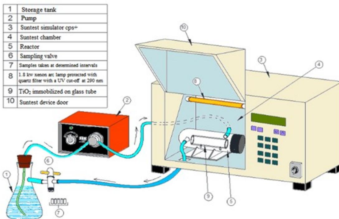
Figure 1. Cooled solar simulator equipped with TiO<sub>2</sub> immobilized on glass tubes.
